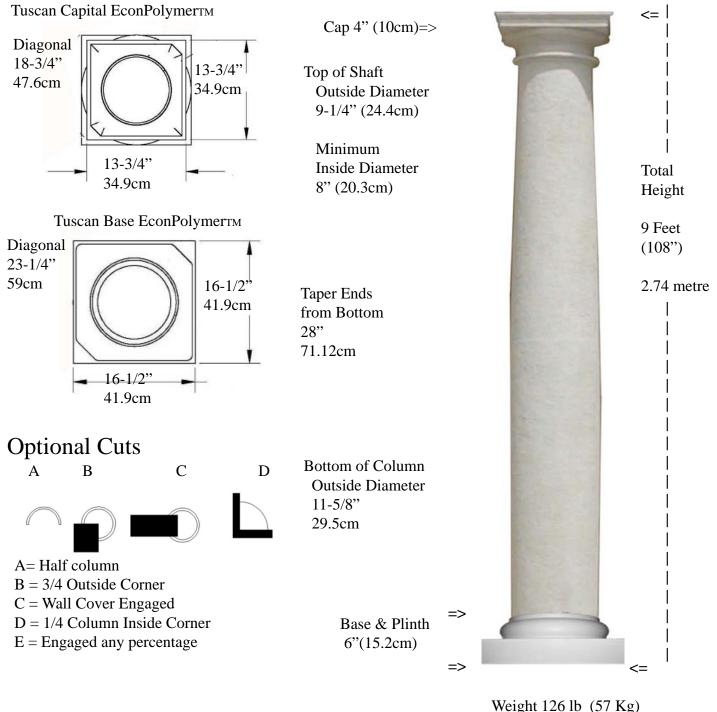
Weight 126 lb (57 Kg) Load o/c to 18,000lbs (8.16m tons)
